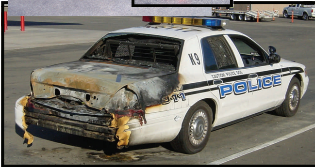
Accidental Combustion of Fuse Flares in Trunk of Police Car
